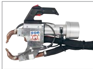
High pressure water cooled X-tong
